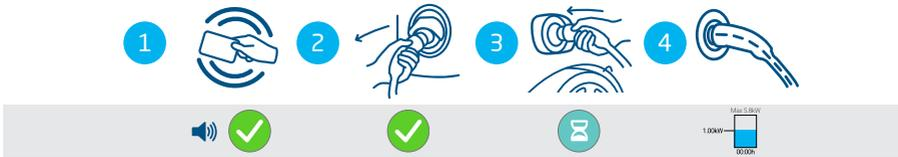
Figure 4.7: Starting the charging process with user authorization / RFID card. Symbols shown on the user interface
