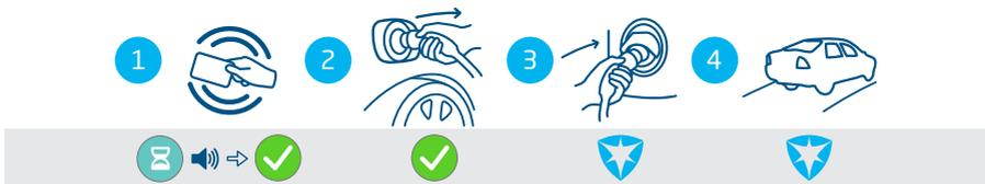
Figure 4.8: Stopping the charging process with user authorization / RFID card. Symbols shown on the user interface
