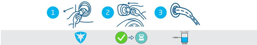
Figure 4.5: Starting the charging process without RFID card. Symbols shown on user interface
