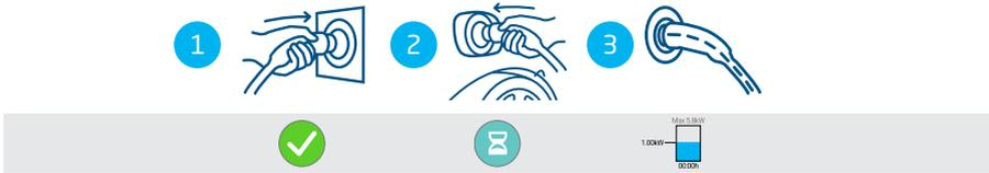
Figure 4.1: Starting the charging process without RFID card. Symbols shown on user interface
