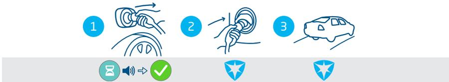
Figure 4.6: Stopping the charging process without RFID card. Symbols shown on user interface
