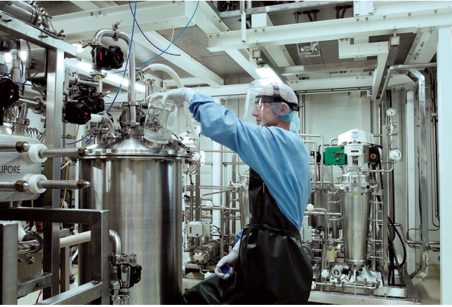
A SynCo manufacturing operator adding cleaning solution to an ultra filtration system
