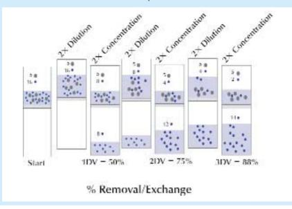
Figure 3: Discontinuous diafiltration (sequential dilution). Large circles represent molecules that are bigger than the pores in the membrane, and small circles represent molecules (such as salts or solvent) that are smaller than those pores.
