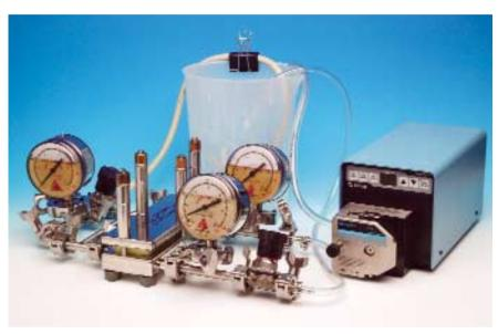
A typical development laboratory system comprising a Centramate holder with a peristaltic pump and pressure gauges, valves, and tubing. PALL CORPORATION (WWW.PALL.COM)
