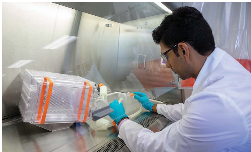
Corning HYPERStack vessels deliver high-density culture of mesenchymal stem cells (MSCs) with optimized gas exchange and a minimal footprint.
