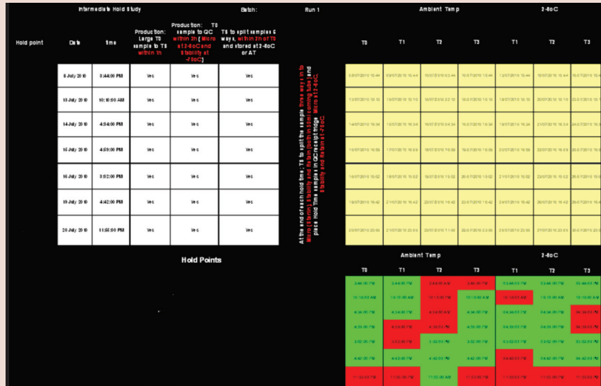
Figure 1: Sample tracking using an MS Excel visibility board. Time zero of each process hold step triggers the spreadsheet to repopulate remaining hold times for that step. Using a visibility board, operators can arrange a daily meeting with all relevant departments to review samples due at the end of a hold period for that day or shift period. Samples due out of hours or during weekends may also be highlighted and are colored red; samples within a working day are highlighted in green. Sample tracking and coordination ensures efficient resource management.
