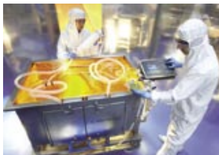
Photo 1: Example of a single-use bag system (SARTORIUS STEDIM BIOTECH, WWW.SARTORIUS-STEDIM.COM)
