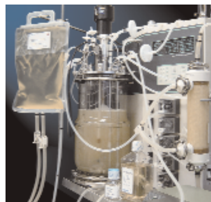
This 12-L bioreactor in perfusion mode using a 0.2- \mu m hollow-fiber cartridge (to culture a GS NS0 transfectoma producing human IgG in HyQ SFM4MAb and HyQ LS250) is being run in the Department of R&PD at HyClone's Logan, UT facility. (HYCLONE, LOGAN UT).
