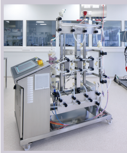
Photo 2: Automated skid for virus filtration
