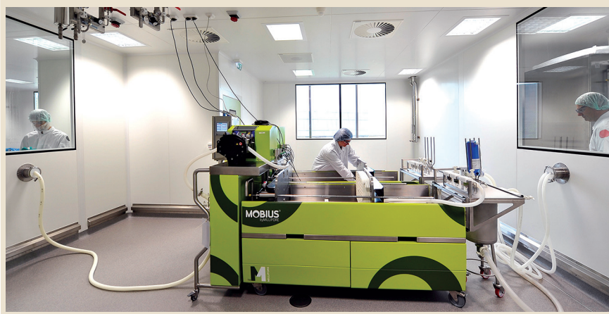
Photo 3: Harvest area; the double skid is designed with adjustable filtration capacity. Disposable input and output tubings are passed through the wall with port holes. Utilities from the ceiling were created to anticipate possible process adaptation requiring cold-recirculation loop, purified water, and compressed air.
