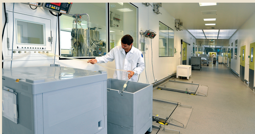
Photo 5: View of the ISO 9 material hall; media or buffers are transferred to the equipment through transfer hatches designed to allow passage of disposable tubing. Media or buffers requiring temperature-controlled storage can be connected to recirculation loops located on the upper wall.
