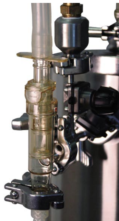
Photo 1: As a critical link between stainless-steel equipment and single-use systems (e.g., bags or tubing sets), Steam-Thru technology creates a contamination-free connection. Made of non-animal-origin, USP Class VI polysulfone with platinum-cured silicone seals, these products can be safely connected to either bioreactors or process skids.
