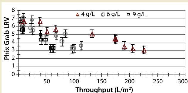
**Figure 5:** Instantaneous LRV as a function of mass loading ( $\text{g/m}^2$ ) for three MAb concentrations tested in triplicate (one lot shown here)
