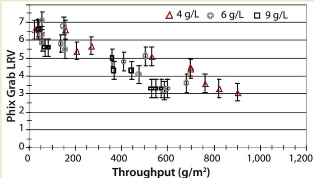
**Figure 6:** Instantaneous LRV as a function of flow decay for three MAb concentrations tested in triplicate (one lot shown here)
