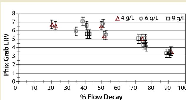
**Figure 7:** Pool LRVs at 75% flow decay for one membrane lot (4, 6, and 9 g/L, respectively) tested in triplicate
