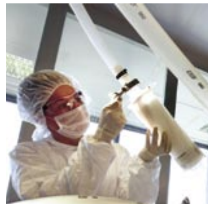
A purification operator handles a single-use 30-inch membrane-based chromatography device.
