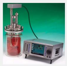
Biomass monitor 220 (Aber Instruments Ltd., UK) for real-time measurement of viable cell concentration. Photograph shows a cell culture application with a top entry electrode.
