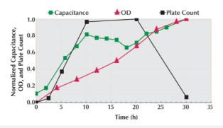
Yeast Monitor can reveal a unique yeast growth and flocculation profile. The capacitance trace not only provides valuable information on the cell concentrations after seeding and transfer to the next stage, but a change in the profile will also provide valuable feedback on any upstream changes in the quality of the media (brewers' wort) feed.
