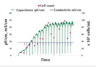
**Figure 10:** Monitoring an Escherichia coli fermentation by RF impedance, optical density, and plate counts in a pilot plant 2,000-L fermentor (units have been normalized).
