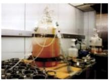
Photo 4: Hybridoma cells cultured in a 50-L polypropylene bioreactor, with a 36-L culture volume (see reference 7 for details)
