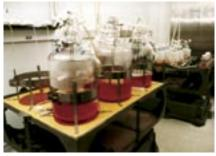
Photo 3: CHO cells cultured in 20-L polycarbonate bioreactors, with a 5-L culture volume
