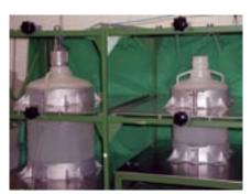
Photo 1: 50-L (left) and 20-L bioreactors mounted on a standard RC-6 shaking machine (Kühner AG, Switzerland). The shaking machine has a fixed shaking diameter of 50 mm.
