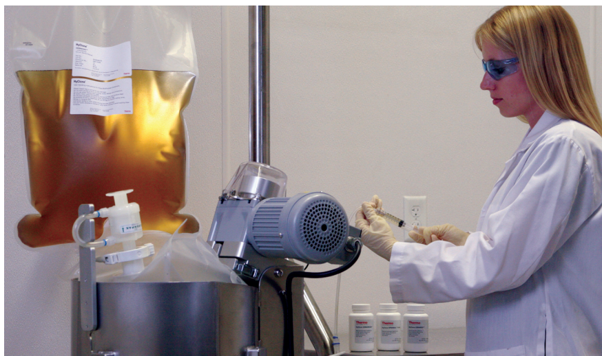
Serum-free medium supports efficient bioproduction in a classically sparged 250-L single-use bioreactor using a pitched-blade impeller
