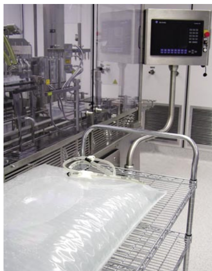
A 100-L disposable biobag (Sartorius AG) in an aseptic suite at Hyaluron
