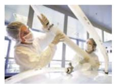
**Photo 1:** Purification associates are handling a 30-in Q membrane chromatography device. It can be used for virus clearance and trace contaminant removal at large scale.
