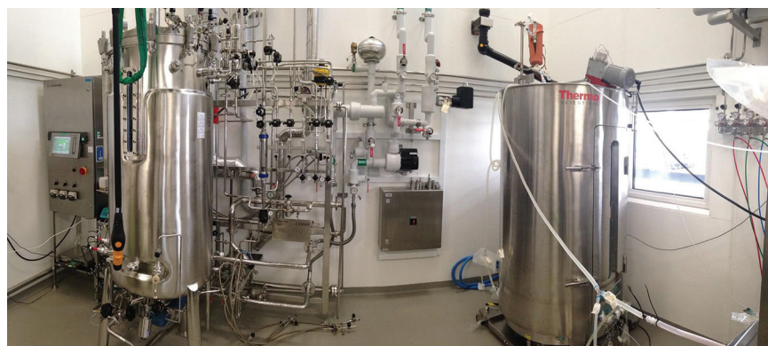
Flexible pilot facility with a 350L stainless steel bioreactor and a 1,000-L single-use bioreactor.
