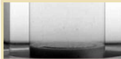
Photo 1: Showing the clarity of packed columns as evidenced by the frit, when the refractive indices of the mobile phase and stationary phase match exactly. Stationary phase: Nucleosil C18, particle size 10 \mu m. Mobile phase: dichloromethane/toluene/cyclohexanol (14%/17.2%/68.8%).
