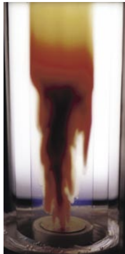
In an extreme case of VF, the band width expands to the column length
