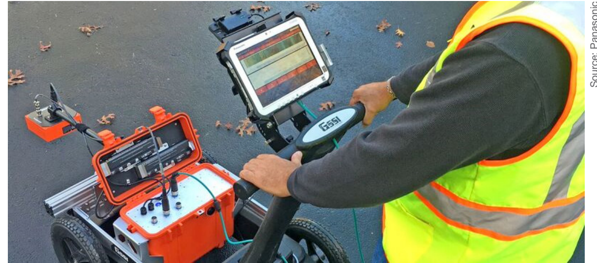
A surveyor uses GSSI's ground-penetrating radar system, which uses a Panasonic Toughpad as its controller platform, to scan a roadway to determine the precise location of underground cables and pipes.
