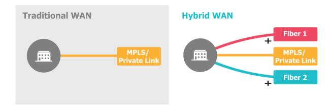
The end result is a Wide Area Network made up of multiple connections between each location that can be actively used at the same time to improve connection reliability and aggregate bandwidth.
