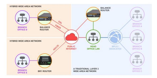
With the simple addition of a couple of static routes on the private WAN and public Internet access routers, the new branch office locations added in this way can communicate securely with both the head office LAN devices as well as the remote branch locations on the traditional WAN.
