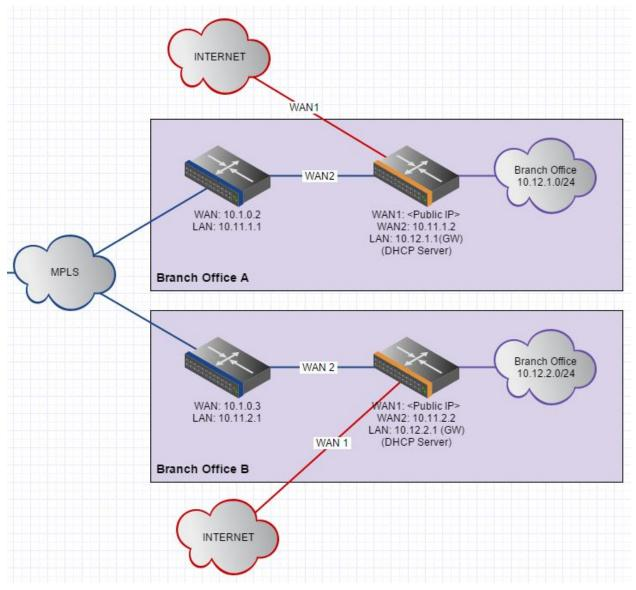
In the remote branch offices a new Peplink Balance router is added to act as the gateway device for the local network and the branch office subnet is changed to be in the 10.**12**.x.0/24 range.
