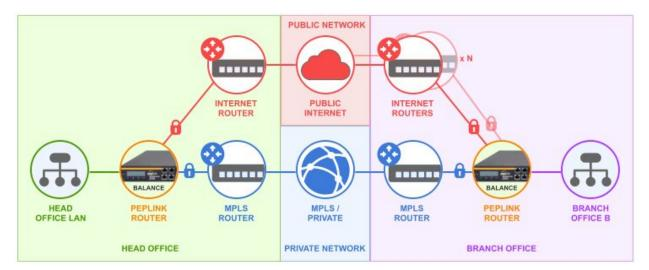
In this example, the head office network now has three routers. A Peplink Balance device has been added to act as the default gateway for the network. This has the public Internet access router and the private WAN access router connected to its WAN ports.
