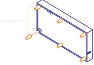
Screw in the connectors to the underside of the bases and use them to mount the two bed bases to each other.
