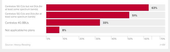
Several options exist for RAN centralization. Full centralization of the baseband components requires fronthaul connectivity with CPRI and eCPRI, but a partial centralization of only the centralized unit (CU) function results in a midhaul transport segment handled by Ethernet. Additionally, some operators are choosing to centralize their 4G RANs along with 5G.
