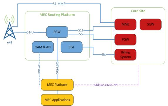
Fig. 4 MEC solution architecture using the SGW-LBO approach
