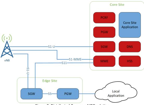
Figure 2. Distributed Core as a MEC solution
