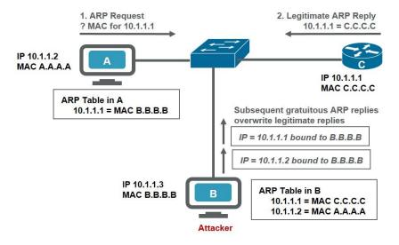
ARP spoofing attacks and ARP cache poisoning can occur because ARP allows a gratuitous reply from a host even if an ARP request was not received. After the attack, all traffic from the device under attack flows through the attacker's computer and then to the router, switch, or host.
