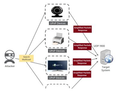
Figure 2: SSDP Flood - DPI software can detect traffic based on SSDP protocols
