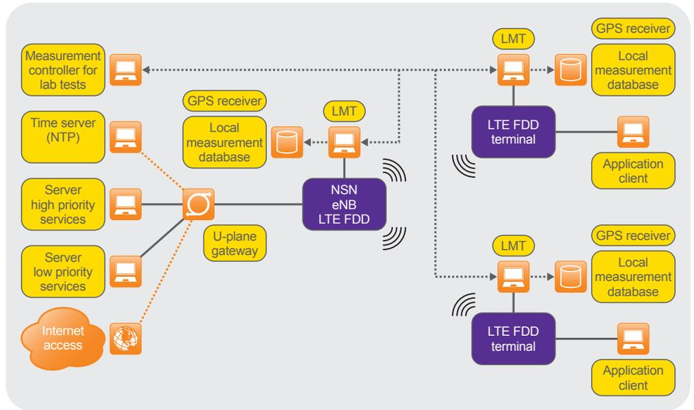
Figure 1. Nokia Siemens Networks LTE development platform
