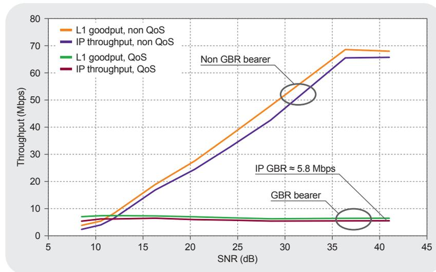
Figure 13. DL tests with different QoS bearers per UE under lab conditions
