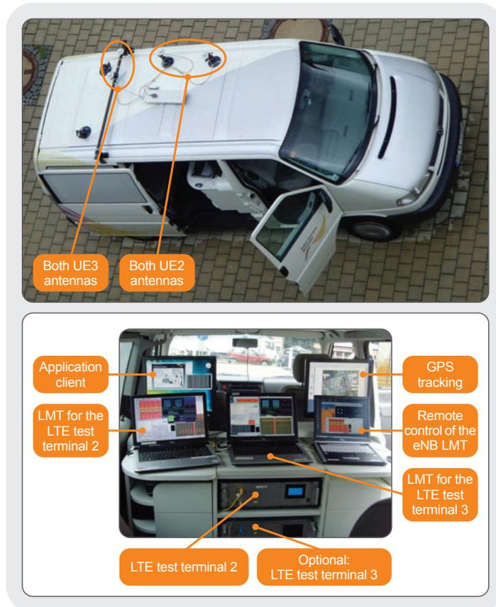
Figure 2. Measurement van with LTE UEs
