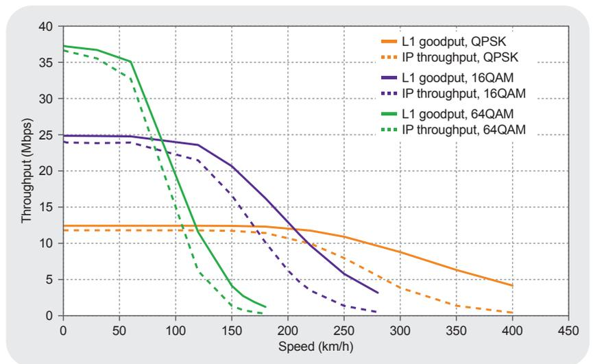
Figure 12. Speed test for SIMO transmission under lab conditions
