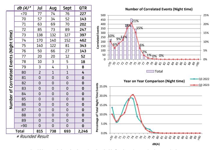
N.B It should be noted that the detection thresholds for the noise monitoring terminals are set at the lowest level to record the maximum number of aircraft noise events. A number of smaller aircraft types, such as business jets and propeller aircraft, get very close to but do not reach the detection threshold.
