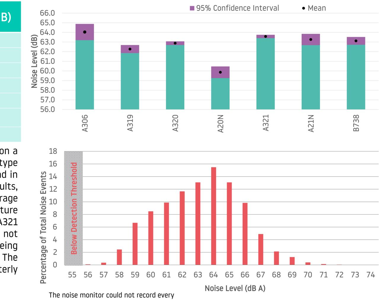
aircraft noise event if the aircraft noise level is below ambient background noise (≤55dB).
