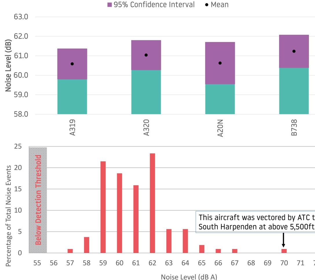
The noise monitor could not record every aircraft noise event if the aircraft noise level is below ambient background noise (≤55dB).
