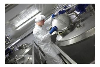
**Picture 1:** PDX Reactor technology was integrated with Mitsubishi Electric equipment to create a 1200kg plant that produces white sauce in a single-stage process.
