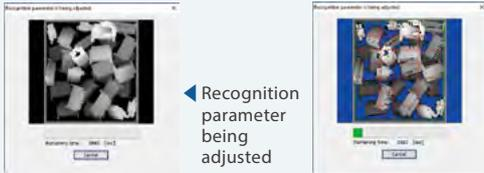
Randomly stacked parts are replicated in a simulation. The most suitable parameter is selected and adjusted.
