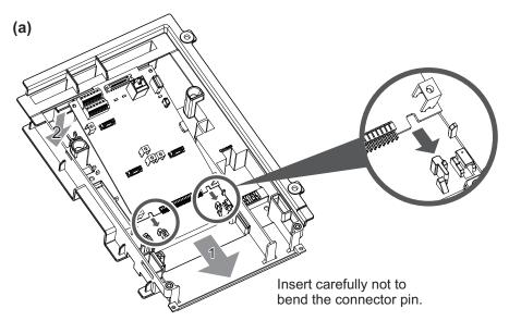
(a) Tilt the control circuit board, fit it into the hooks of the base unit, then lay it flat.
