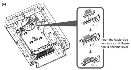
(e) Connect the cable to the connector of the control circuit board and the connector on the upper right of the base unit. Route the cable through this hook.
