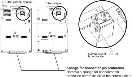
the base unit. Use care not to bend pins of the connector.
