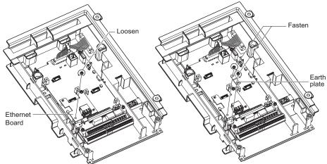
(f) Remove the mounting screw on the bottom left of the Ethernet board before installing the Ethernet board earth plate to the base unit.
