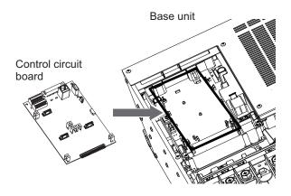
Install the control circuit board according to the following steps.
