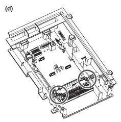
(d) Tighten the screws on the control terminal block unit to fix it to the base unit.
