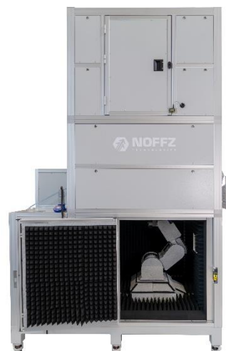
NOFFZ Universal Tester Platform UTP tests and calibrates radar sensors that are used in automotive applications, for example.
