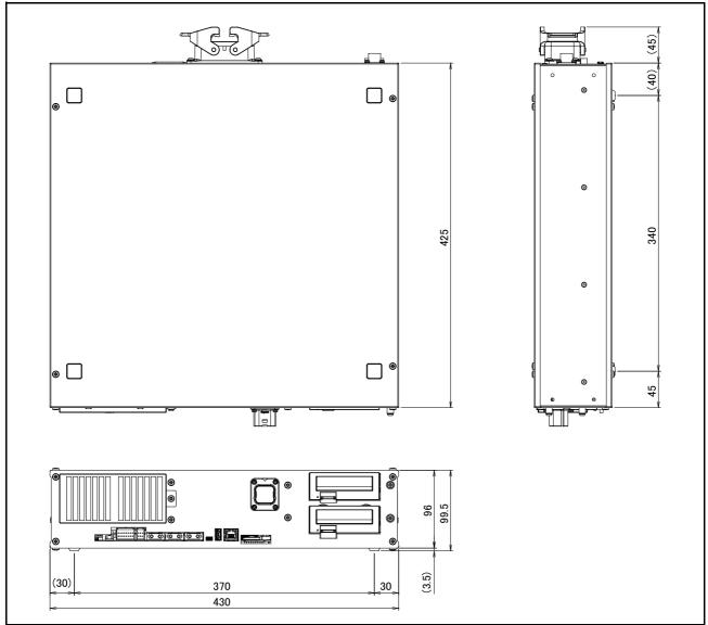
Fig.3-2: Outside dimensions of controller
