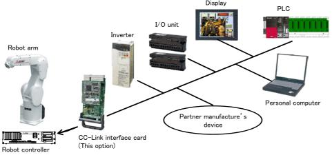
Fig.3-37: Example of CC-Link Product Configuration
