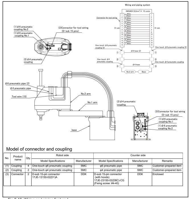
Fig.2-16: Wiring and piping for hand
