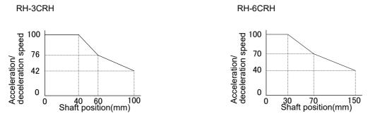
Fig.2-6: Relationship Between Offset Amount and Maximum Speed
