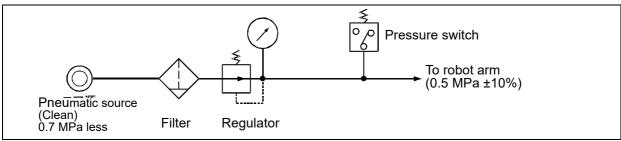
Fig.2-19: Air supply circuit example for the hand
