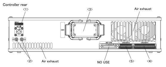
Fig.3-1: Names of controller parts
