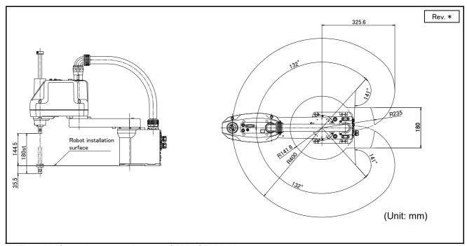
Fig.2-11: Operating range diagram of RH-3CRH4018
