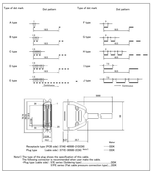
Fig.3-36: Connections and outside dimensions
