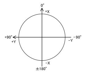
Fig.4-1: Definition of component C for conventional robots (within ±180)
