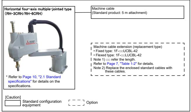
Fig.1-1: Structural equipment
