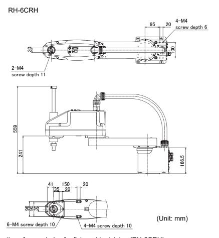
Fig.2-18: Location of screw holes for fixing wiring/piping (RH-6CRH)
