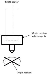
Fig.4-3: Origin position adjustment
