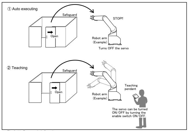
Fig.3-11: Door switch function
