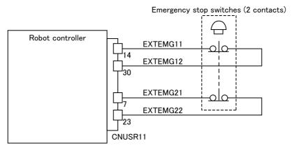
Fig.7-2: How to wire emergency stop lines
