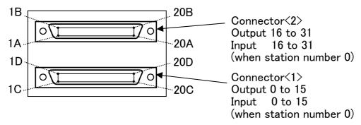
Fig.3-22: Pin layout of connector
