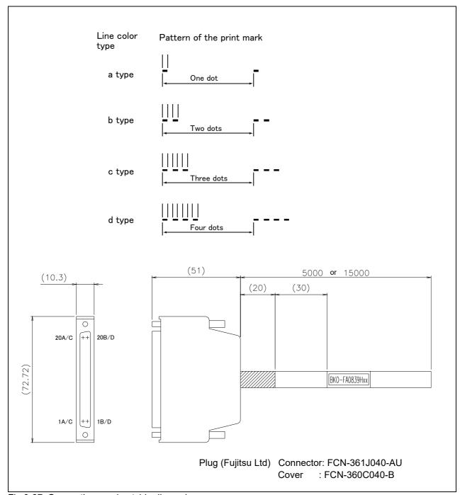
Fig.3-27: Connections and outside dimensions
