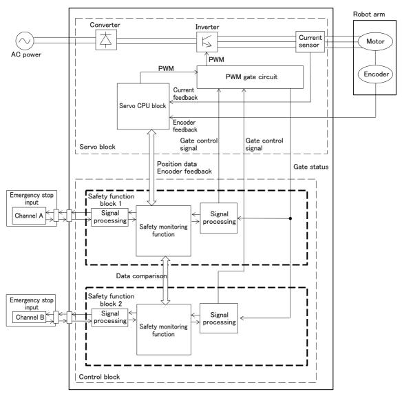
Fig.7-3: Safety block diagram
