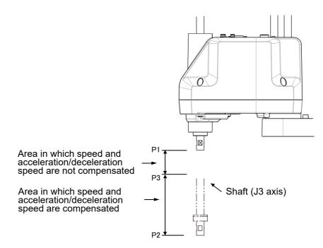
Fig.2-4: Area in which acceleration/deceleration speed is compensated
