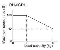
Fig.2-3: Automatic compensation of speed
