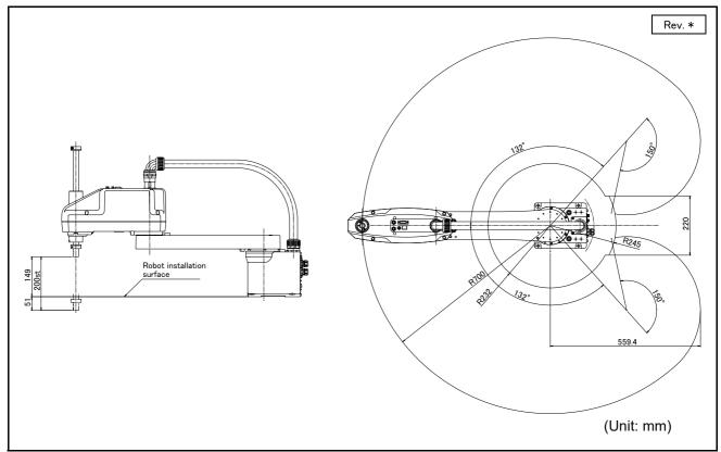
Fig.2-15: Operating range diagram of RH-6CRH7020
