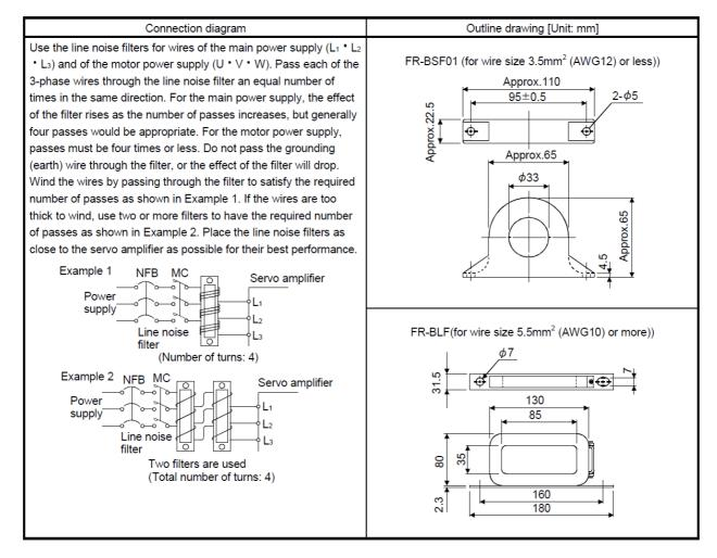
Fig.3-15: Example of noise filter installation
