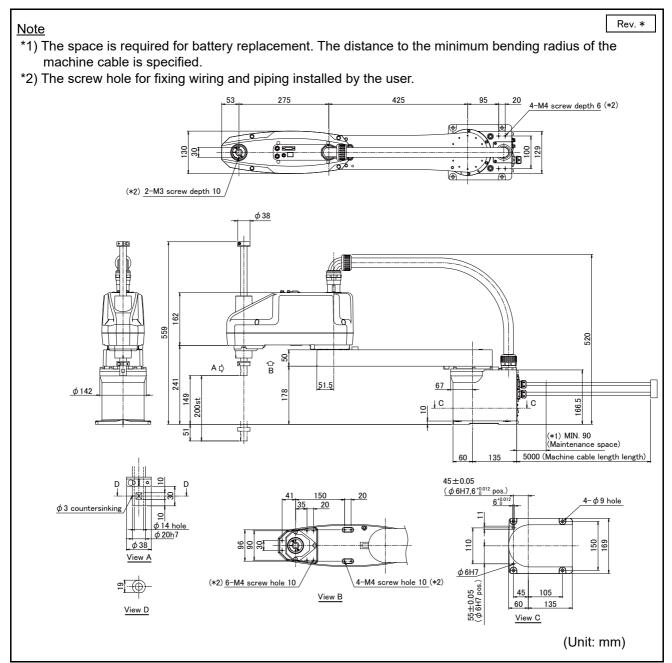
Fig.2-14: Operating range diagram of RH-6CRH7020
