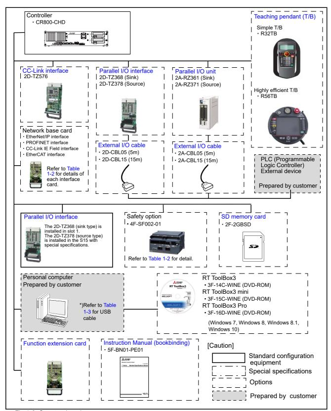
Fig.1-2: Structural equipment
