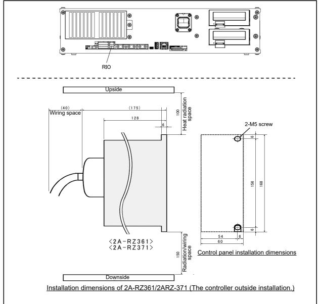
Fig.3-29: Installing the parallel I/O unit
