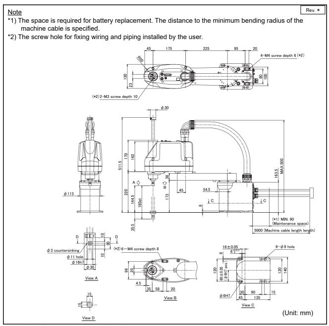
Fig.2-10: Outside dimensions of RH-3CRH4018
