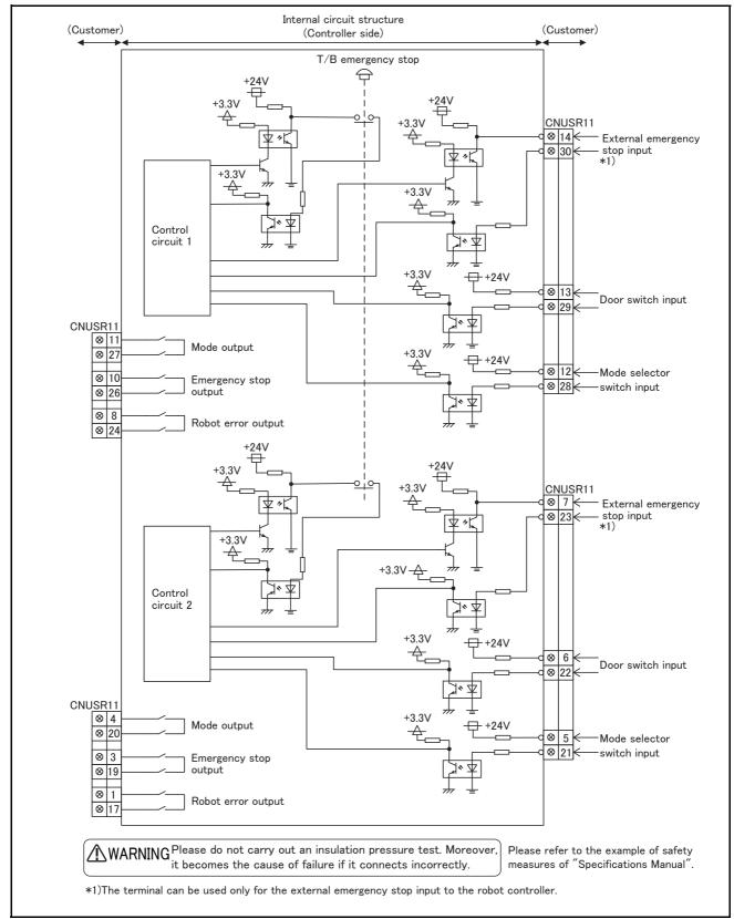
Fig.3-8: External emergency stop connection
