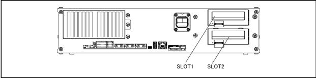
Fig.3-21: Parallel I/O interface installation position
