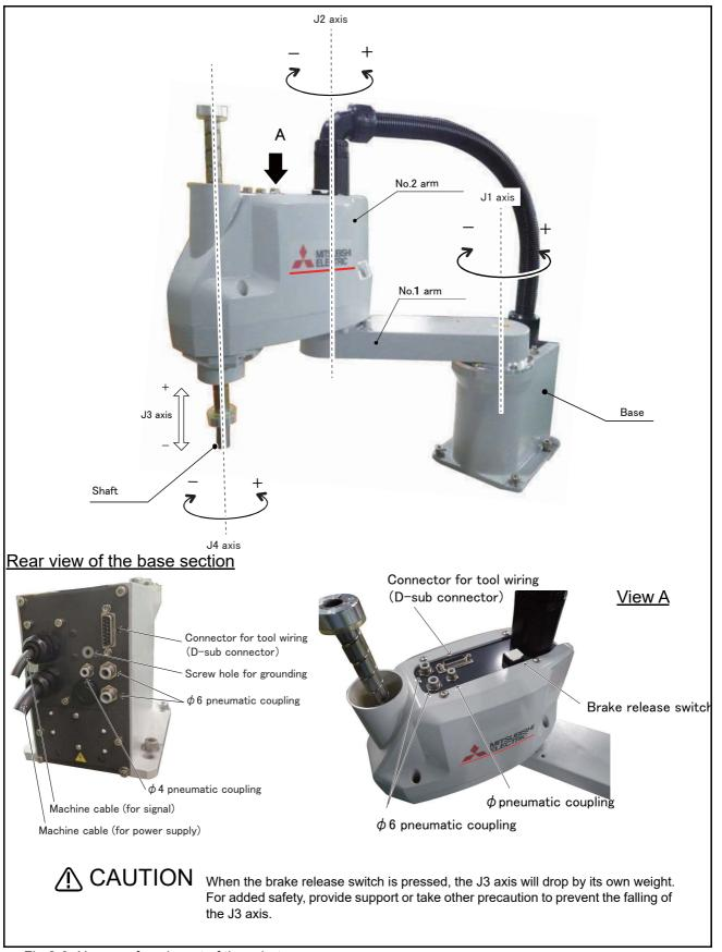
Fig.2-9: Names of each part of the robot
