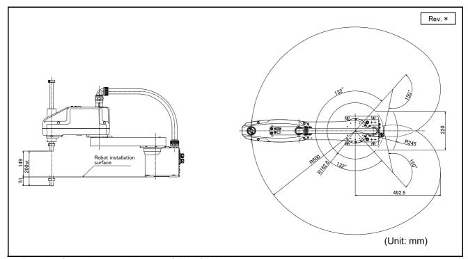
Fig.2-13: Operating range diagram of RH-6CRH6020
