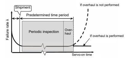
Fig.2-21: Periodic inspection/overhaul periods
