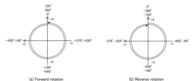
Fig.4-2: Definition of component C for RH-3CRH/RH-6CRH (over ±180)
