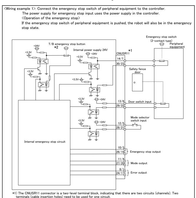
Fig.6-1: Example of safety measures (wiring example 1)
