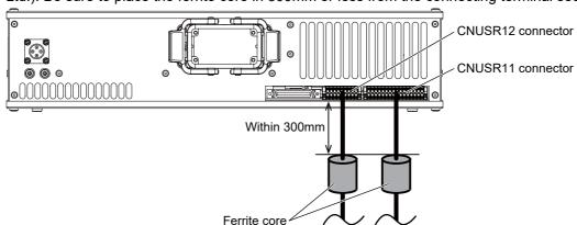
Fig.3-6: Installation position of ferrite cores
