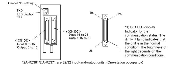
Fig.3-31: Pin arrangement of the parallel I/O unit
