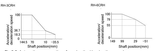
Fig.2-5: Automatic compensation of acceleration/deceleration speed
