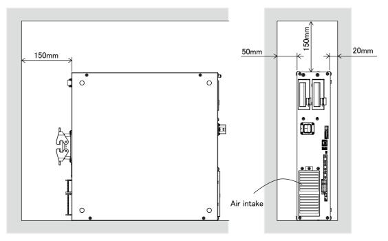
Fig.3-3: Installation dimensions
