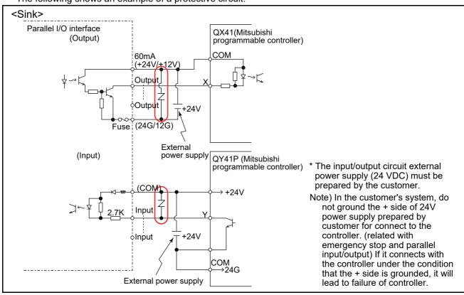
Fig.3-24: Connection with a Mitsubishi PLC (Example of sink type) for use of a protective circuit
