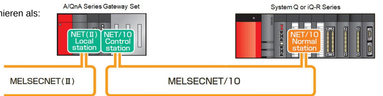
Step-by-step replacement with System Q or iQ-R Series
