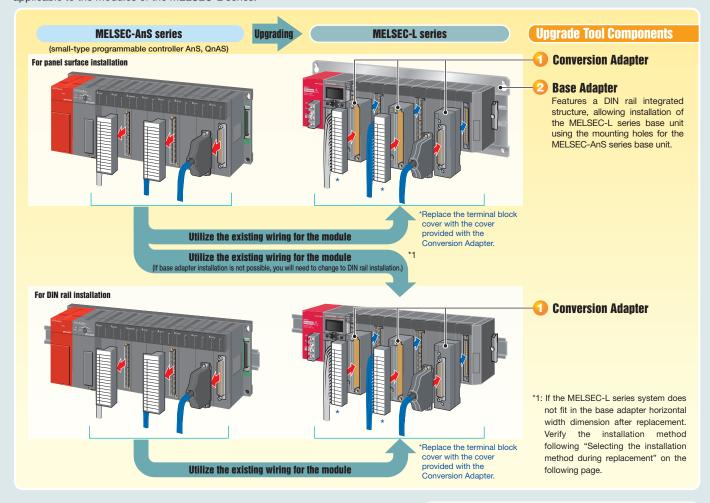
If you replace a terminal block type module, the wiring may interfere with an adjacent module. Use of the Mitsubishi Electric LG69 space module is recommended.
