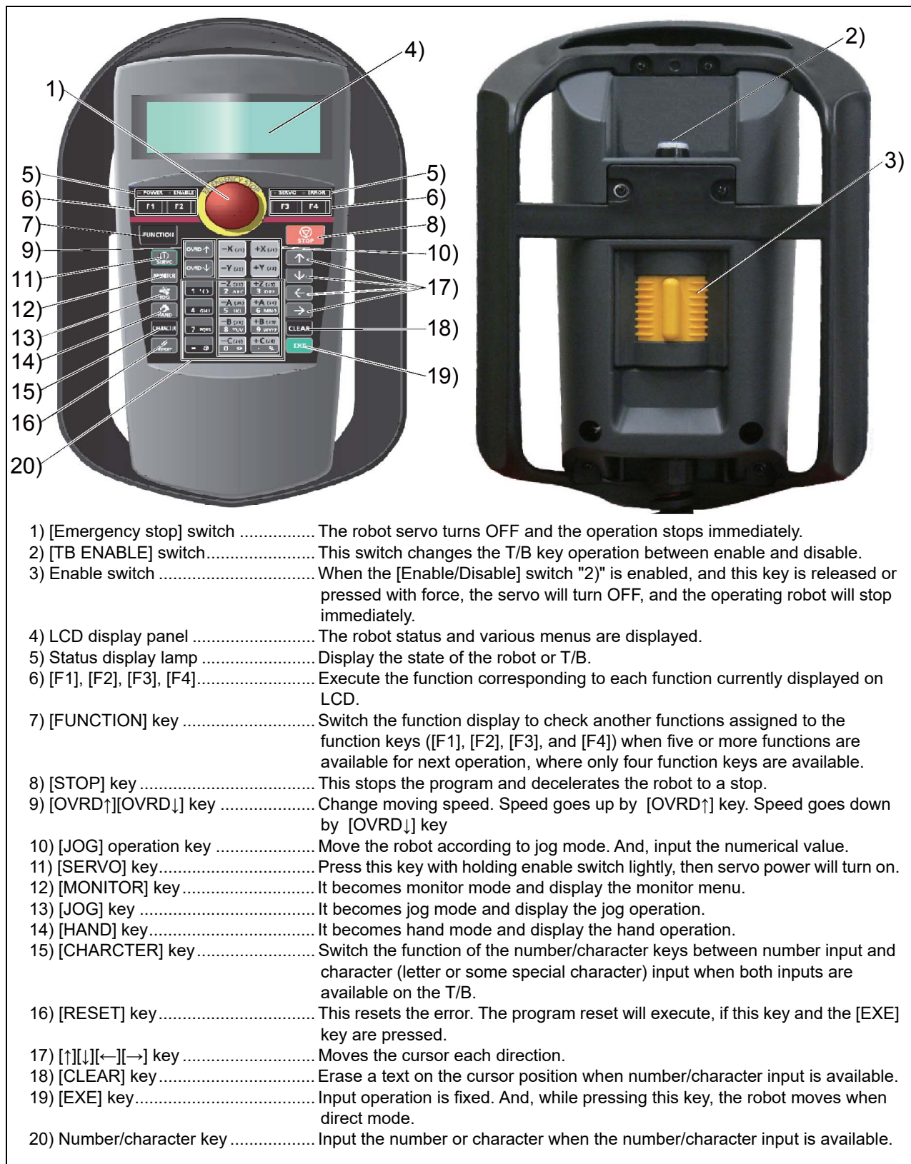
Fig.3-19: Teaching pendant key layout and main functions
