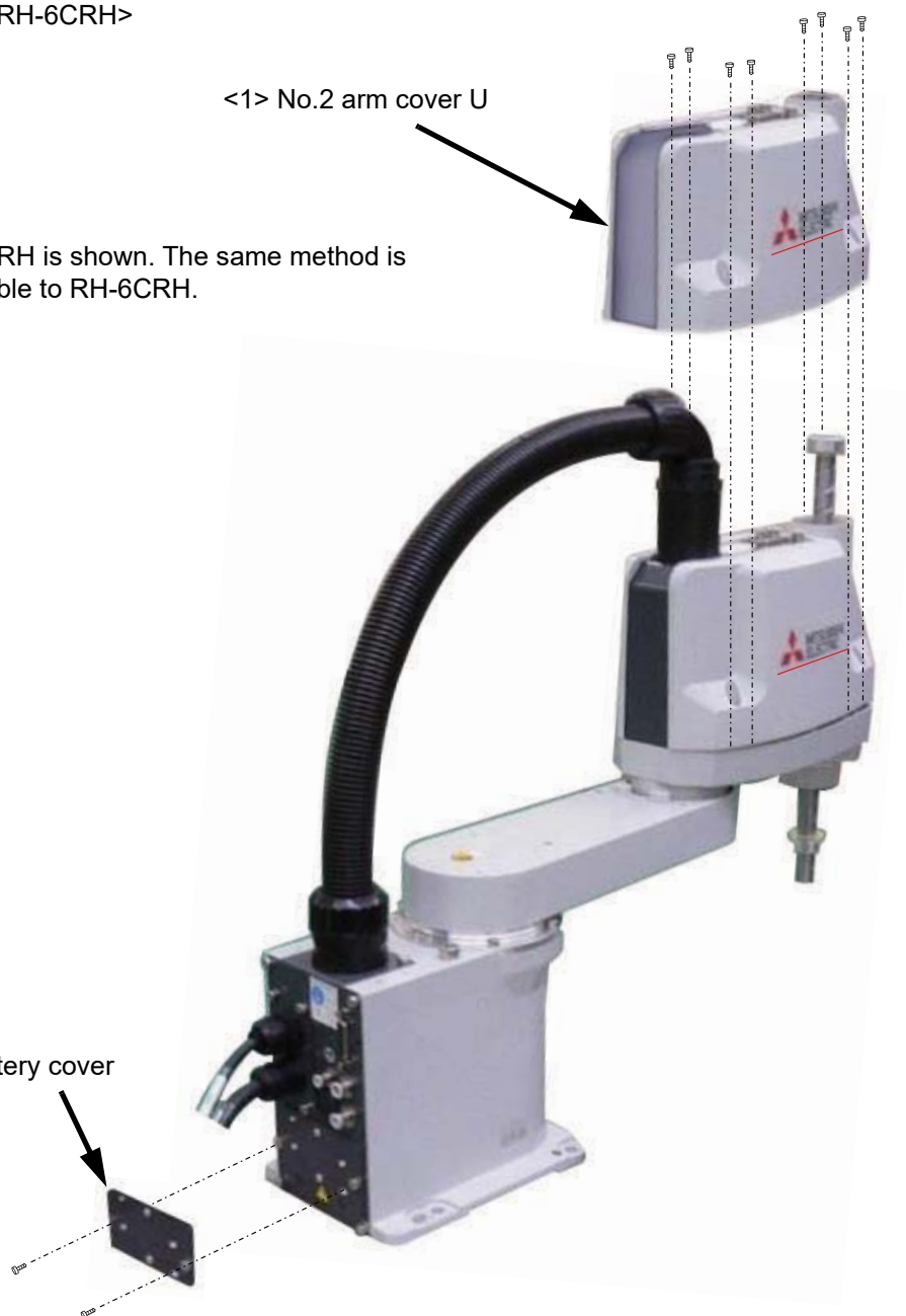
Fig.5-2:Installing/removing the cover (RH-3CRH, RH-6CRH)
