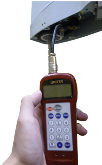
Fig.5-3:Tension adjustment method of timing belt
