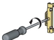
4. Loosen the screw on DIN rail stopper.
