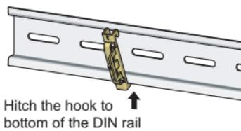
5. Hitch the bottom hook of the DIN rail stopper to the bottom of the DIN rail. Check the orientation of the DIN rail stopper according to the arrow on the front of the stopper.
