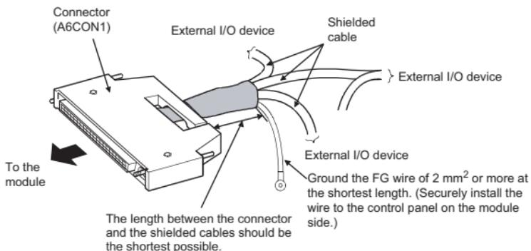
[Example of processing for a shielded cable]
