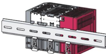
3. Lock the DIN rail hooks to the DIN rail to secure the modules in the position.
