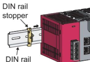
7. Slide the DIN rail stopper to the leftmost module.
