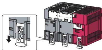
1. Pull down DIN rail hooks on the back of the modules until they click.
