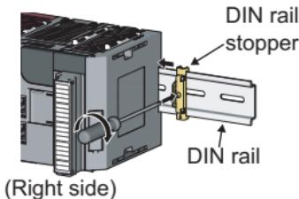
9. Attach a DIN rail stopper on the right of the module with the same procedure.
