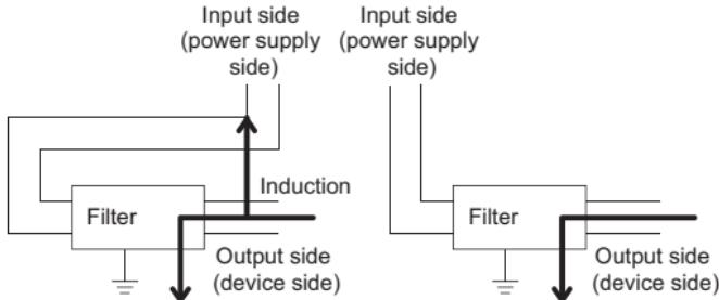
Noise will be induced when the input and output wires are bundled.
