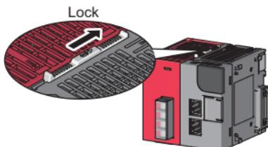
1. To release the module joint levers located at the top and bottom of the head module:
