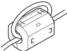
(b) Noise filter (power supply line filter)
