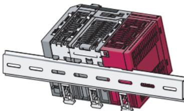
2. Hang the upper tabs of the modules on a DIN rail, and push the modules in position.
