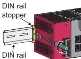
8. Tighten the screw on the DIN rail stopper with a driver.
