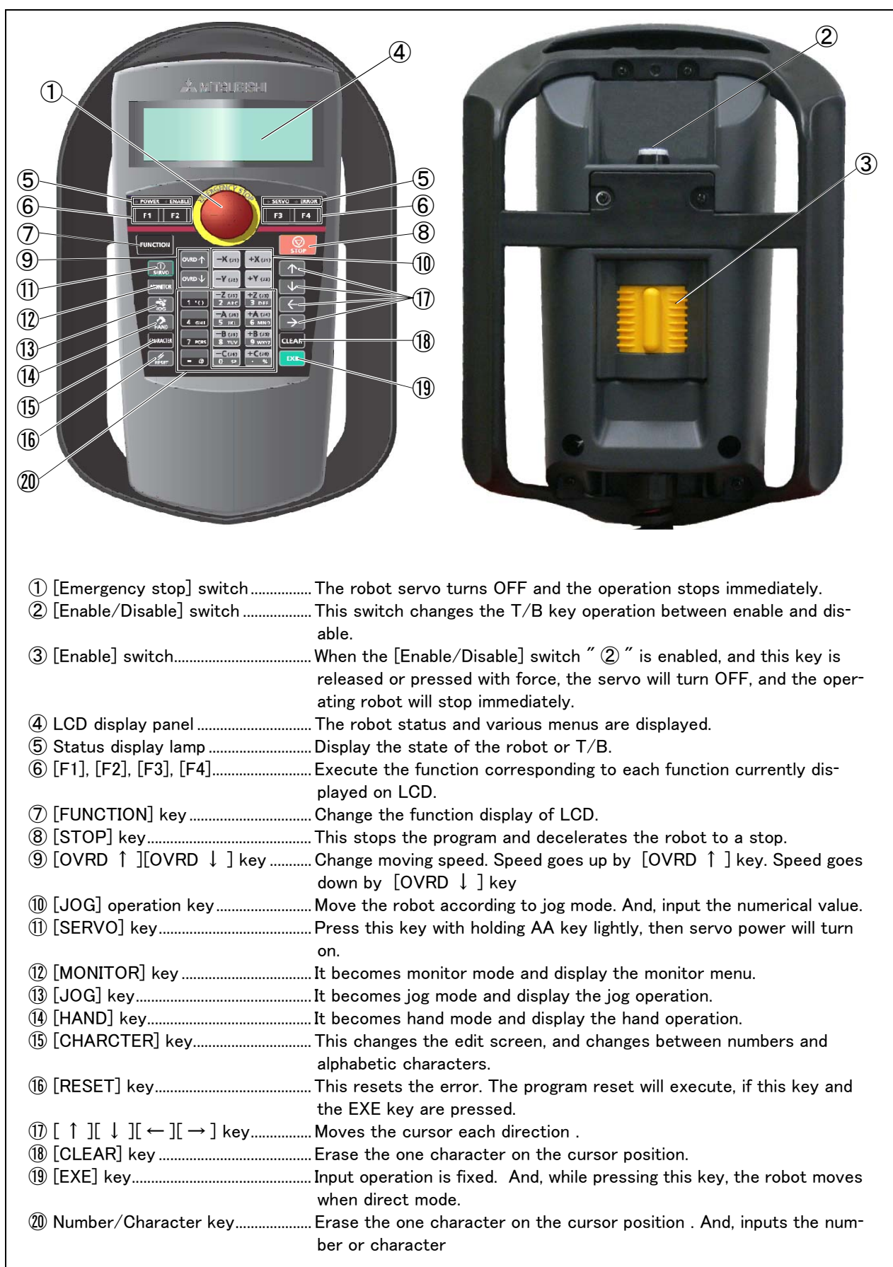
Fig.3-26 : Teaching pendant key layout and main functions
