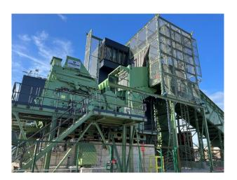
**Image 1:** Existing metal recycling systems can easily be retrofitted with low-maintenance variable frequency inverters with three-phase induction motors, resulting in savings on energy, wear and maintenance costs.
