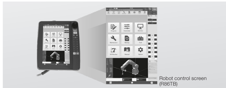
Enables automatic operation of servo motor on/off, startup and shutdown, reset, program selection, and other operations.
