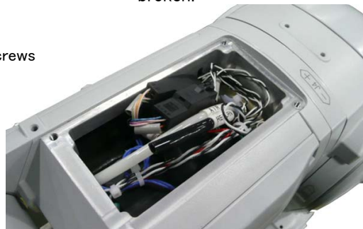
The condition of storing the cable inside the No.2 arm cover U
