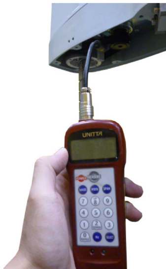
Fig.5-7 : Tension adjustment method of timing belt
