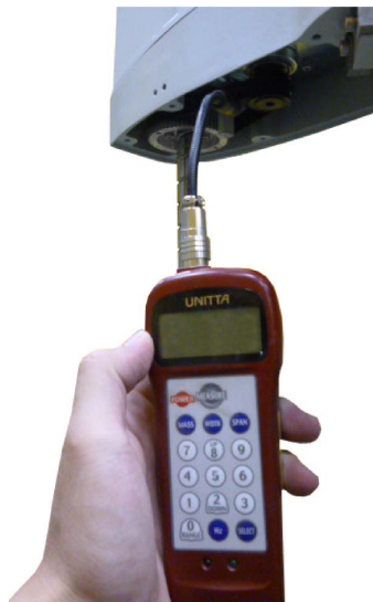
Fig.5-7 : Tension adjustment method of timing belt
