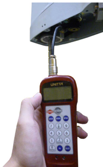
Fig.5-7 : Tension adjustment method of timing belt
