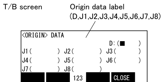
Fig.5-34 : Correspondence of origin data label and axis
