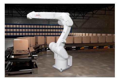
[Source: Mitsubishi Electric Europe, Germany] Image caption: Mitsubishi Electric's latest MELFA RV-12CRL vertical articulated robot supports industrial automation pick-and-place applications with a 1,504 mm reach and 12 kg payload capacity.
