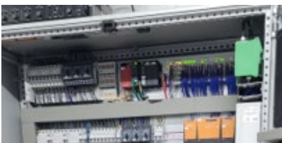
Pic 6: The MELSEC System-Q PLC control system manages all simulator functions
