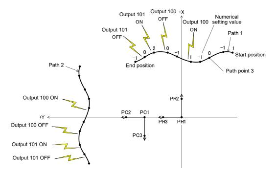
Fig.7-103:Movement of sample program
