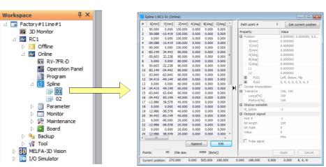
Fig.7-44:Opening a spline file saved in the controller
