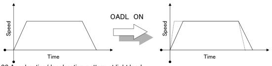
Fig.4-36:Acceleration/deceleration pattern at light load
