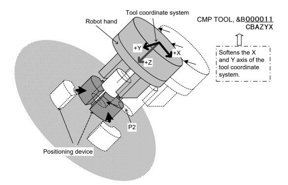
Fig.4-19:The example of using the compliance mode
