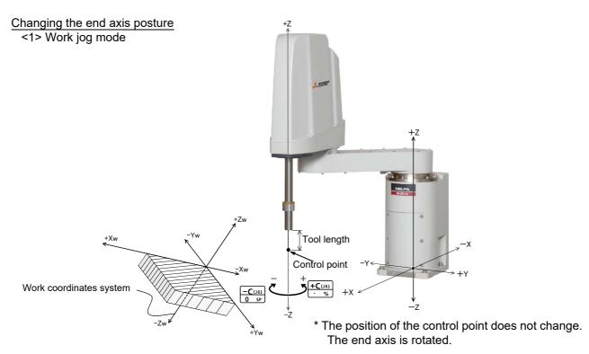
• When the[+C (J6)] keys are pressed, the Z axis will rotate in the plus direction of the XYZ coordinate system.
