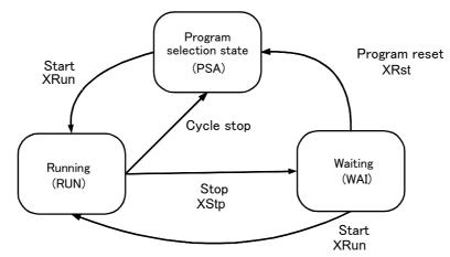
Fig.4-2:Operation state of each slot
