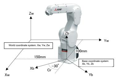
Note) The figure is an example of a vertical 6-axis robot. In horizontal 4-axis robot is the same. (Example)
