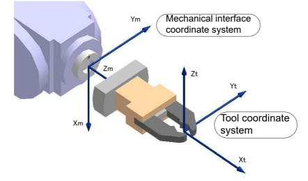
Fig.4-12:Mechanical interface coordinate system and tool coordinate system
