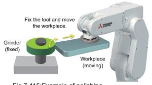
Fig.7-115:Example of polishing
