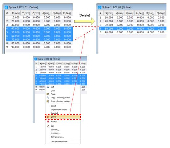
Fig.7-55:Deleting the path point data
