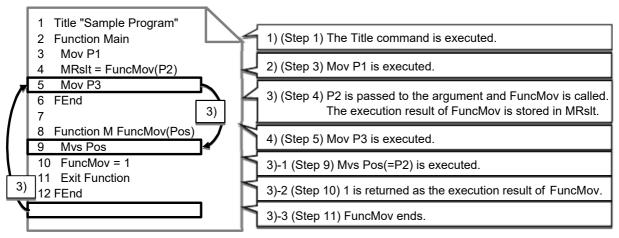
Fig.4-5:Flow of processing with the Function procedure
