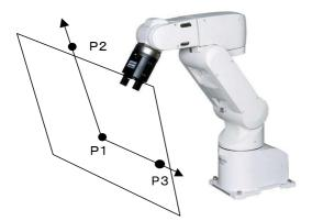
As can be seen in the diagram to the left, any plane can be defined by three points (P1, P2, and P3), after which an evaluation of which side of the plane it is in (the side that includes the robot origin or the other side) can be performed. This function can be used to prevent collision with the floor or interference with peripheral devices. Maximum of eight planes can be monitored. There is no limit to the plane.
