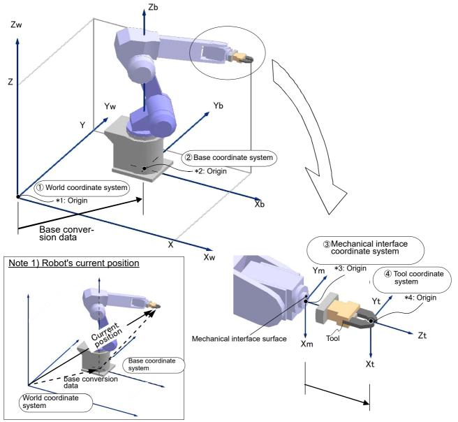
Fig.4-7:Robot's coordinate system
