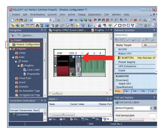
Fig.6-1:GX Works3 module configuration screen (one robot)
