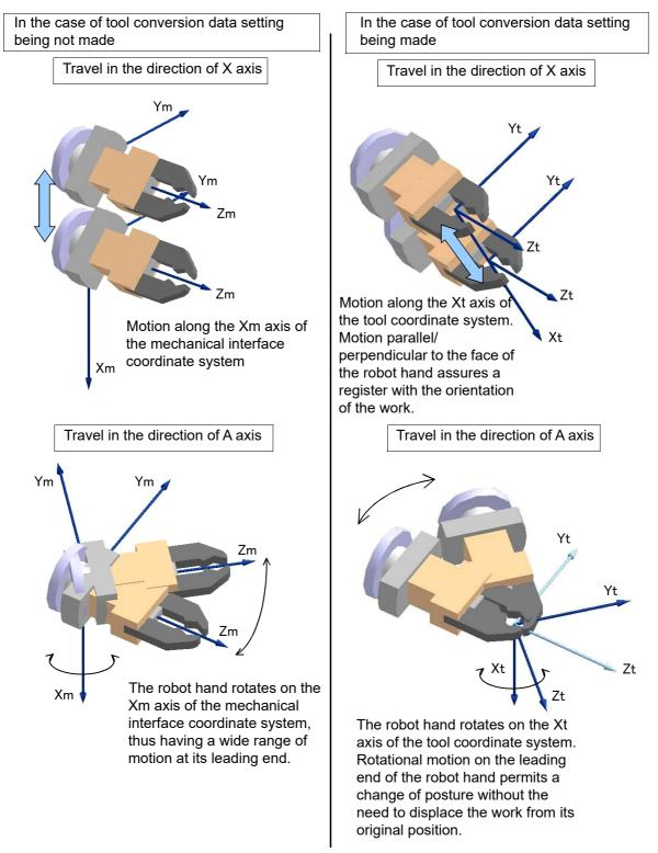
Fig.4-13:Tool jogging operation with/without tool conversion data
