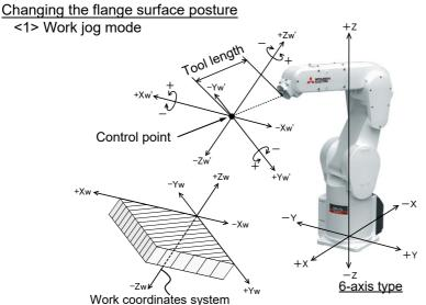
\* The position of the control point does not change. Change the direction of the flange in accordance with the work coordinates system.
