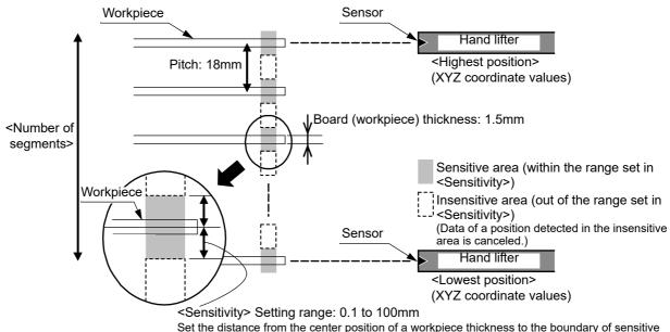
Set the distance from the center position of a workpiece thickness to the boundary of sensitive and insensitive areas.
