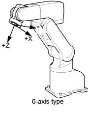
Definitions of Coordinate Axes The tool coordinate is used for the coordinate axes. Axes that must be set:
