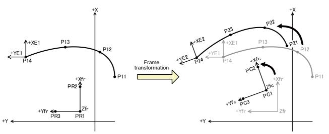
Fig.7-23:Frame transformation (Ex-T spline interpolation)
