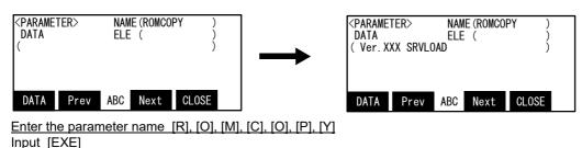
2) Press the function key ([F1]) corresponding to "DATA" to display the parameter input screen. Press the [EXE] key on the parameter input screen.
