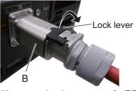
When removing the connector for T/B connection, use lock release (state which raised the lock lever to the up side), make the case of the B section slide to the front, and remove and pull up out the latch.
