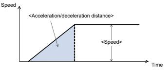
Fig.4-35: Acceleration with <Acceleration/deceleration distance>
