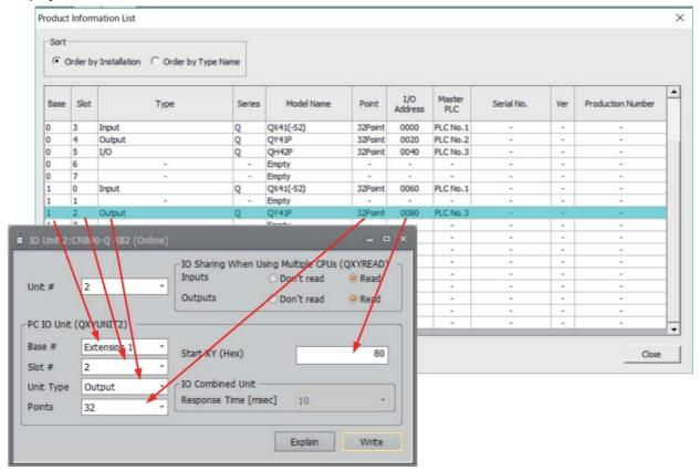
After setting the above parameters, reset the power of the PLC and robot CPU.
