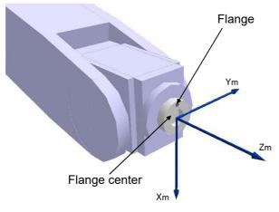
Fig.4-10:Mechanical interface coordinate system
