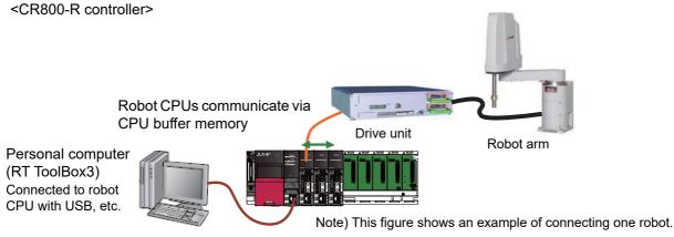
Fig.5-14:Connecting the devices (CR800-R controller)
