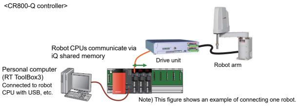
Fig.5-15:Connecting the devices (CR800-Q controller)
