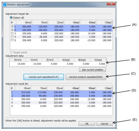
Fig.7-105:Position adjustment screen
