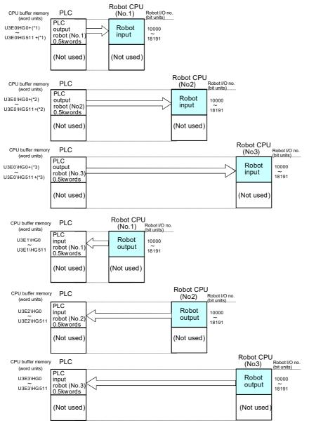
The following figure shows the memory map for the CR800-R series. For the CR800-Q series, refer to the Table 5-4 and replace the device numbers with the corresponding device numbers in the figure.
