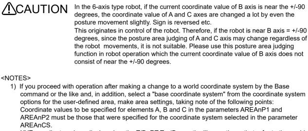
XYZ coordinate values displayed on the T/B, RT ToolBox or the like are those that refer to the world coordinate system. Thus, when "base coordinate system" is selected in the parameter AREAnCS, coordinate values appearing on the display differ from those to be specified.
