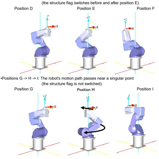
**CAUTION** When passing near a singular point, the robot may rotate in a wide circle as in the case of position H in the figure above. Be sure to keep an eye on the robot and avoid getting in the way when working near the robot, such as when teaching positions.
