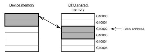
Fig.4-42:Preventing data inconsistency of 32-bit data
