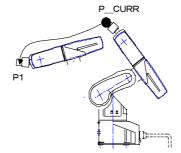
Fig.4-25:Example of joint interpolation motion path
