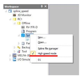
When the high speed spline interpolation command is enabled, high speed spline interpolation is applied to "path point check" and "calculate maximum speed" (shown in Table 7-11). The path point check window will be displayed as shown below.
