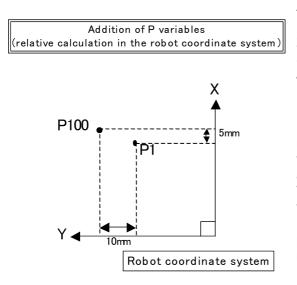
An example of relative calculation(Addition) 1 P2=(5,10,0,0,0,0)(0,0) 2 <u>P100=P1+P2</u> 3 Mov P1 4 Mvs P100 P1=(200,150,100,0,0,45)(4,0)
