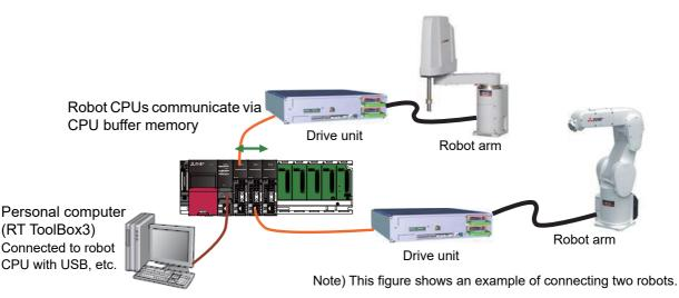
Fig.5-11:Connecting the devices (CR800-R controller)
