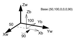
Fig.4-16:Conceptual diagram of the base coordinate system
