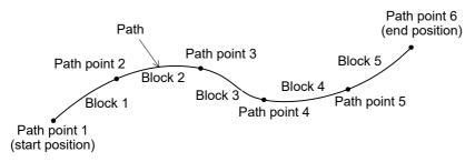
Fig.7-9:Spline interpolation terminology
