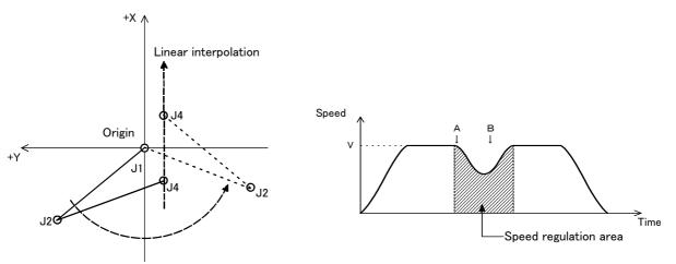
Fig.4-38:Passing through near the origin point
