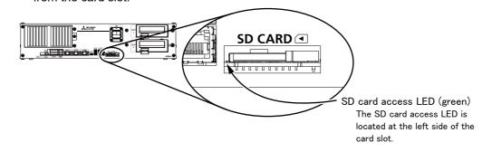
CAUTION The lock state set by the LOCK switch of the SD memory card is ignored in the CR800 controller. Even if the lock state is set, information is written to the SD memory card.
