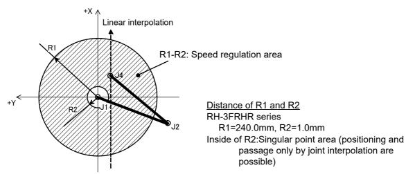
Fig.4-40:Speed regulation area and singular point area
