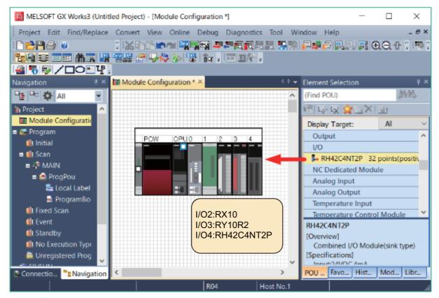
Arrange the input module, output module, and I/O combined module to be used.
