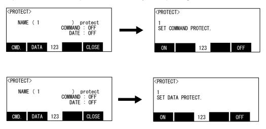
If the function key corresponding to "ON" is pressed, it will be set up for "protecting." If the function key corresponding to "OFF" is pressed, it will be set up for "not protecting."
