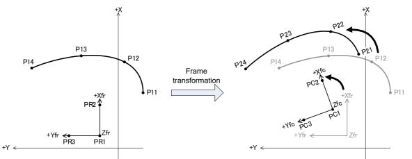
Fig.4-37: Example of frame transformation
