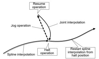
Fig.7-12:Behavior during halt and resume
