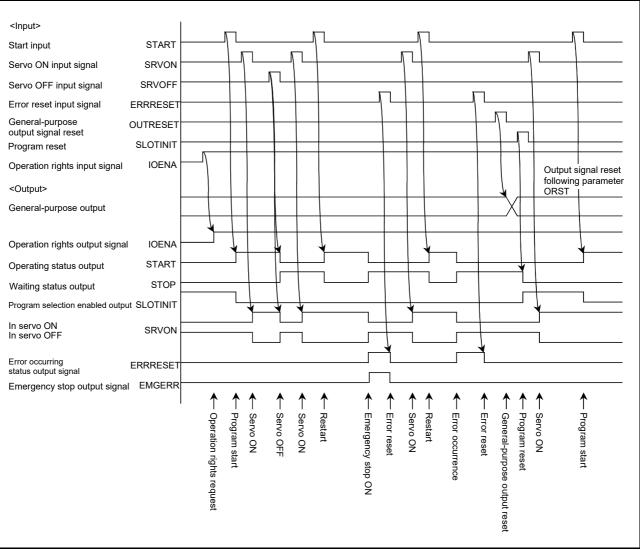
Fig.6-7:Example of external operation timing chart (Part 3)
