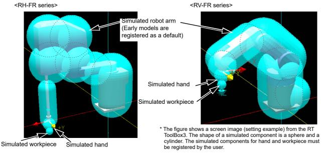
Fig.5-16:Example of simulated component registration
