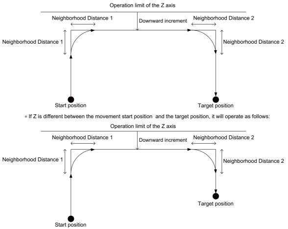
Fig.4-27:Example of Mva2 instruction motion path (seen from the side)
