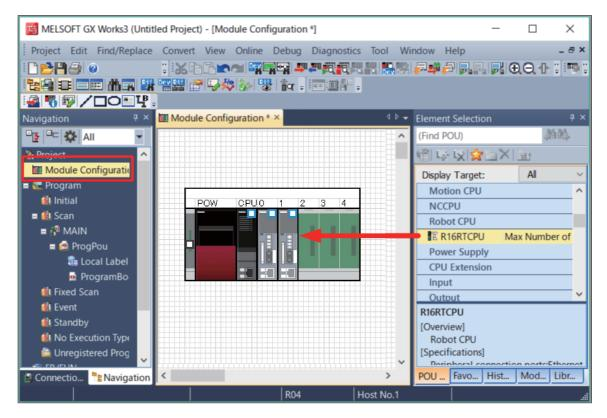
Arrange the extension base, input module, output module, and I/O combined module to be used.
