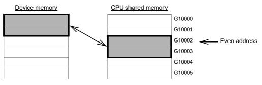
Fig.4-41:Preventing 32-bit data separation
