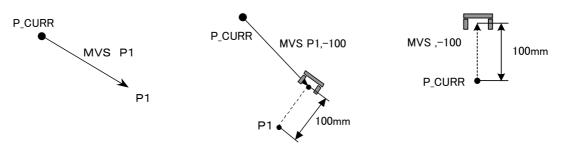
Fig.4-33:Example of movement at linear interpolation
