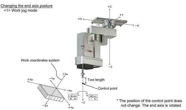
• When the[+C (J6)] keys are pressed, the Z axis will rotate in the plus direction of the XYZ coordinate system.
