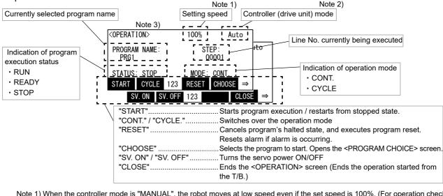
Note 1) When the controller mode is "MANUAL", the robot moves at low speed even if the set speed is 100%. (For operation check) Note 2) When the controller mode is "AUTOMATIC", the T/B's status display lamp [ENABLE] blinks to indicate that the T/B is enabled. The T/B is disabled when the <OPERATION> screen is ended.
