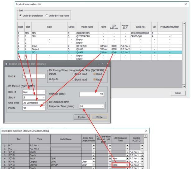
Set "Response Time" according to the value on the window that is displayed by clicking the "Detailed Setting" button in "Q Parameter Setting".
