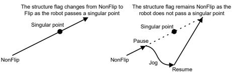
(8) If the singular point passage function is specified, the operation speed may be lowered compared to normal linear interpolation, etc. Moreover, the singular point passage function may affect the execution speed of programs as the function involves complicated processing. Specify the singular point passage function only for interpolation instructions where the function is required.
