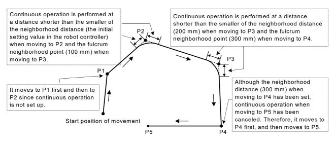
Fig.4-20:Example of continuous path operation
