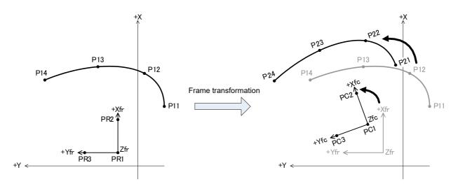
Fig.7-22:Frame transformation (Spline interpolation)
