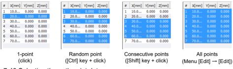
Fig.7-48:Selecting the path point data
