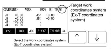
[JOG] Press the key and display the jog screen. ("JOG" is displayed on the screen bottom)
