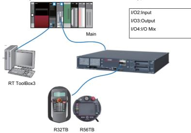
\*System configuration example 2: 2 robot CPUs + 3 types of I/O modules + extension base (added)
