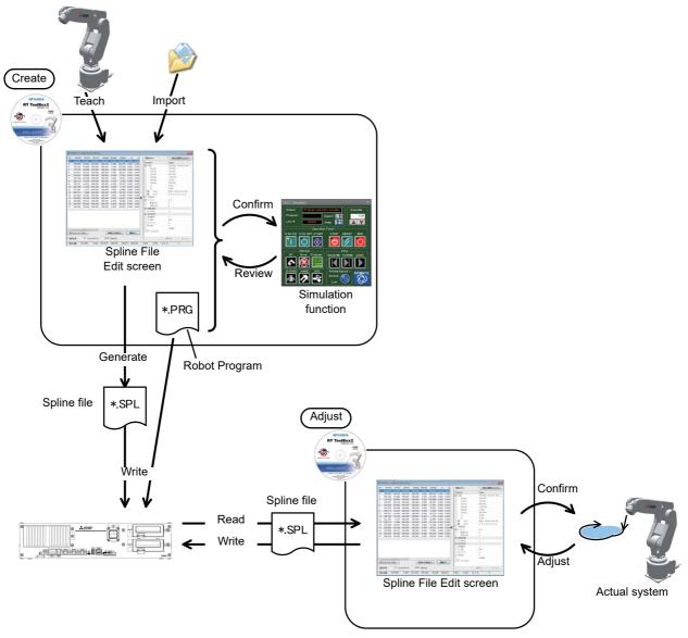
Fig.7-24:Schematic diagram of work details
