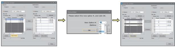
Fig.7-74:Change the spline No.
