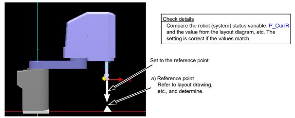
Fig.5-25:Checking the setting for calibration between robots
