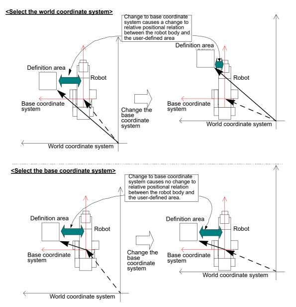
Fig.5-3:Difference between "World coordinate system" and "Base coordinate system"
