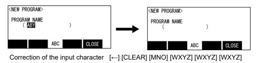
If the long pushing [CLEAR] key, all the data in the parenthesis can be deleted.
