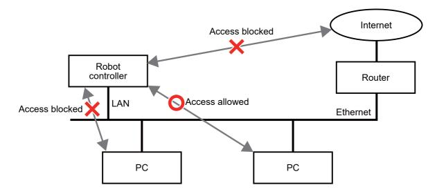
Two access limiting methods, "transparent" and "block", are available. Enable the parameters shown in Table 5-48 to limit the IP address range for filtering. For details on parameters, refer to Page 515, "5.5 Communication parameter".
