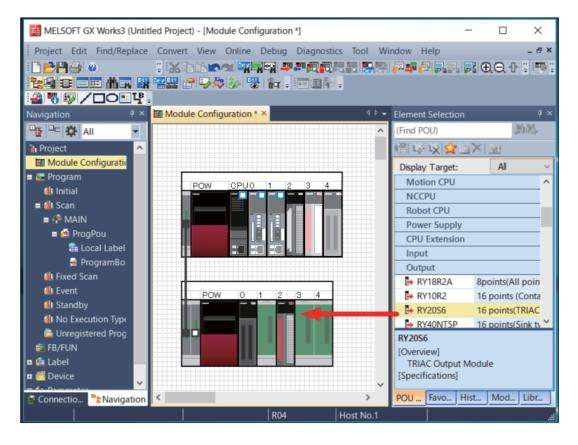
5-600 Direct control of the PLC input/output module
