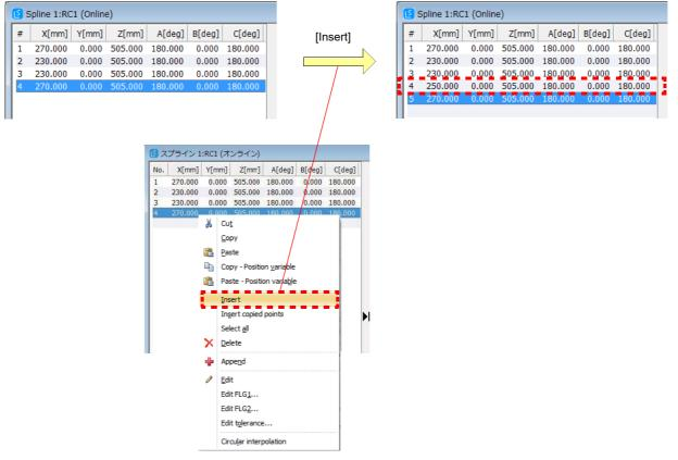
Fig.7-53:Inserting path point data
