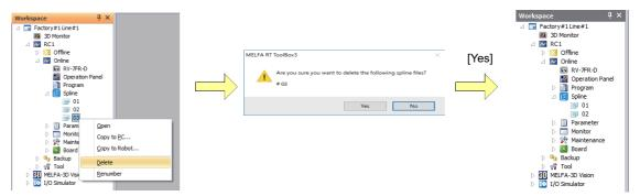
Fig.7-66:Deleting a spline file
