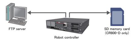
Robot information at error occurrence can be saved in the FTP server or SD memory card (CR800-D only). The following four types of robot information can be saved.
