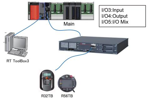
\*System configuration example 2: 2 robot CPUs + 3 types of I/O modules + extension base (added)
