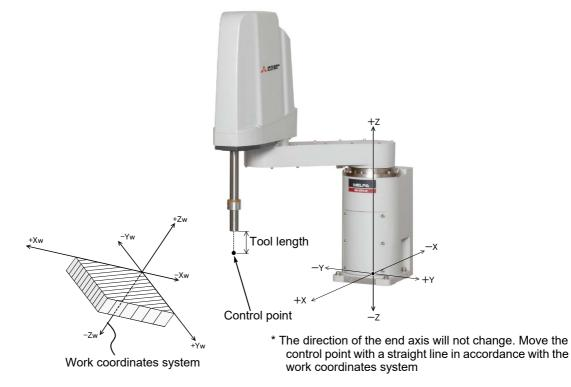
• When the[+X (J1)] keys are pressed, the robot will move along the X axis (Xw) plus direction on the work coordinates system.
