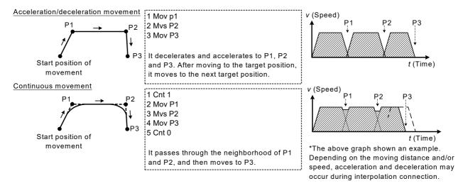
Fig.4-21:Acceleration/deceleration movement and continuous movement
