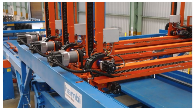
Six grippers lift the structural steel mesh, while servo drives from Mitsubishi Electric move it in all three spatial directions
