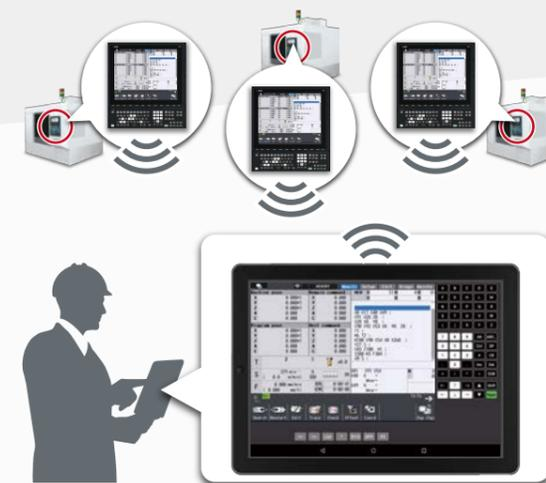
Wireless LAN connection, Screen mirroring to tablet
