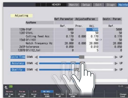
Parameter adjustment screen for high-accuracy control
